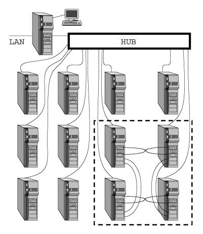
Figure 2: Figure showing the 2-d network torus interconnecting 4 nodes within the PC farm
