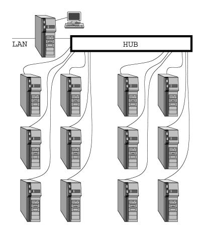
Figure 1: Figure illustrating the PC farm and front end connected to both the LAN and hub
