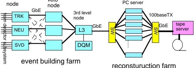
based on PC-servers(4CPU/Linux) connected via Fast/Gigabit Ethernet
