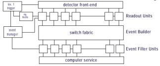
Figure 1 - A typical modern DAQ block diagram
