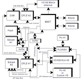
platform for a fully interactive remote develop-download-debug cycle through TCP/IP. The FPGA part is PCI-compliant, so that the custom connector may become a second PCI bus port.
